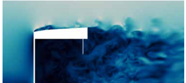
Aerodynamic flow over a balloon launch building for the MET Office - DES Simulation
