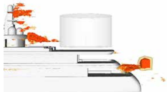
Aerodynamic study of a motor yacht helideck - DeVoogt Naval Architects
