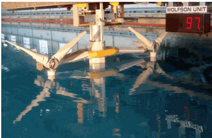
Marine Current Turbines (MCT) model testing
