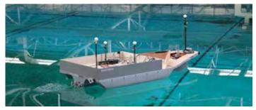
Manoeuvring trials on a 24m SWATH Trimaran designed by AUSTAL Pty
