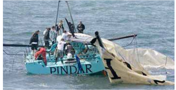
CFRP mast failure investigation
