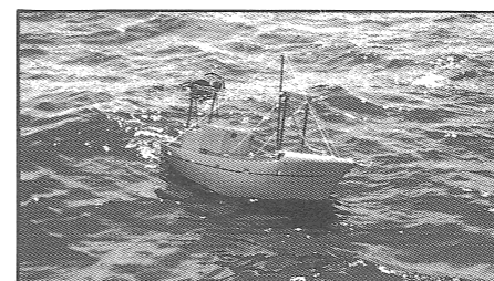
B. Port gear snagged on the bottom, starboard gear on deck, starboard derrick raised. Tension being taken up on the trawl warp.
