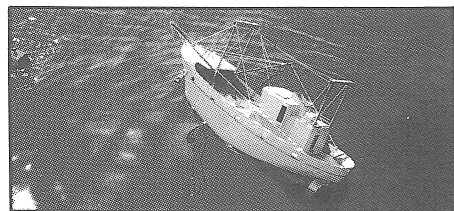
A. Starboard gear snagged on the bottom, port gear (represented by a weight) raised to bulwark height with the port derrick lowered. Tension being increased in the trawl warp.
