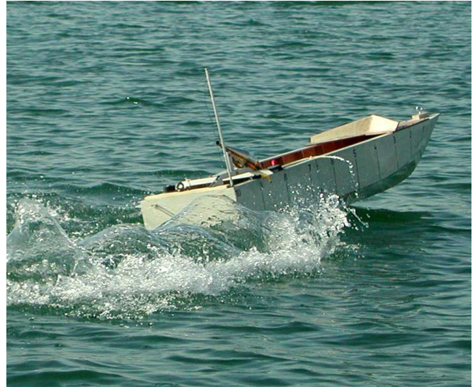
Figure 6 Twin water jet patrol boat under test at 50 knots
