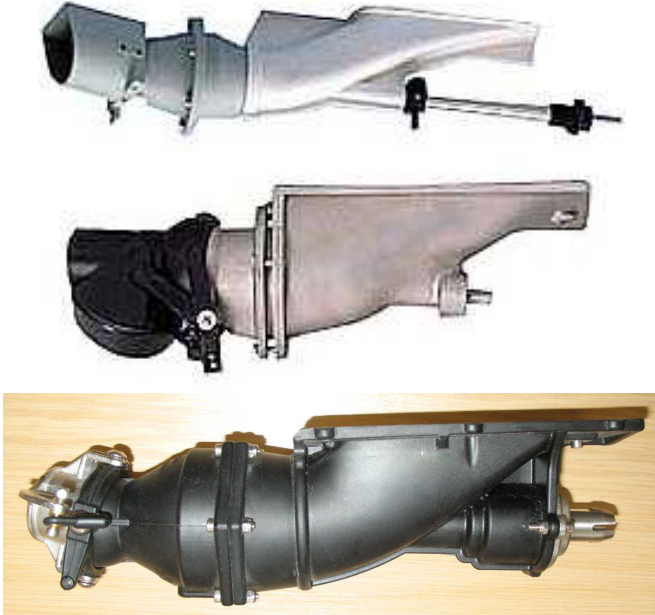
Figure 2 A progression in water jet manufacture: upper jet 0.5kW, mid jet 1kW, lower jet 4kW
