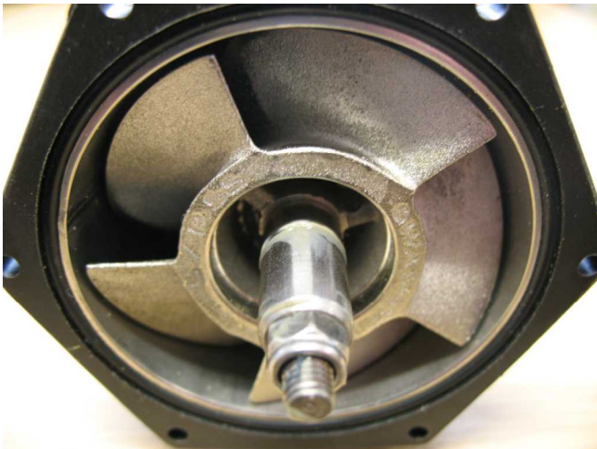
Figure 3 Titanium jet impeller of 50mm diameter
