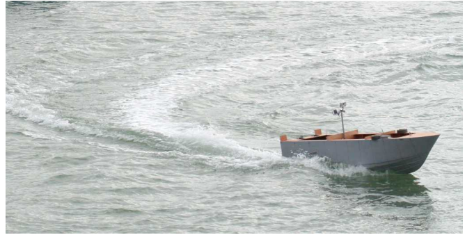
Figure 13 Model of a 26m motor yacht turning at 30 knots
