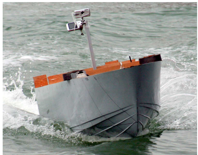
Figure 12 Two compact cameras mounted on a mast for on-board video recording
