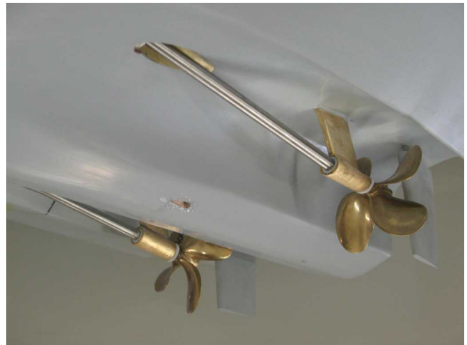
Figure 1 Twin screws in tunnels on a 30 knot motor yacht
