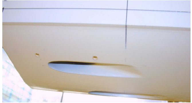
Figure 4 Intakes on a triple jet installation
