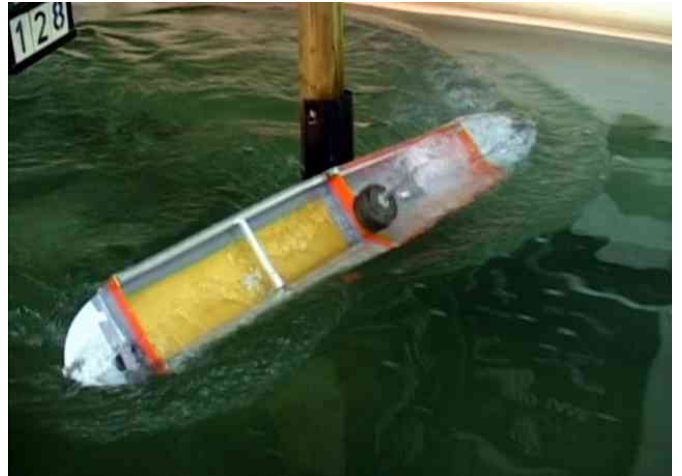
Figure 14. Narrow vessel, with full superstructure, 5.5 knots, 6.4 seconds after impact
