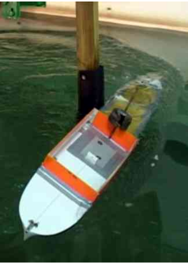
Figure 15. Narrow vessel, with aft superstructure, 4.5 knots, 6.4 seconds after impact
