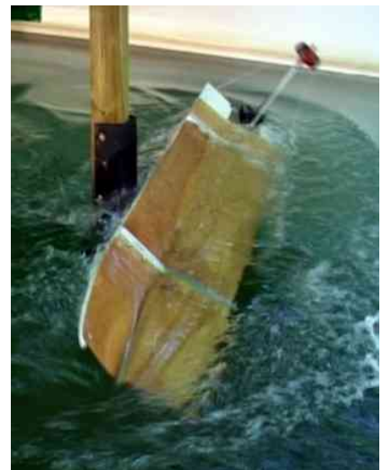
Figure 19. Catamaran, 6 knots, 3.6 seconds after impact
