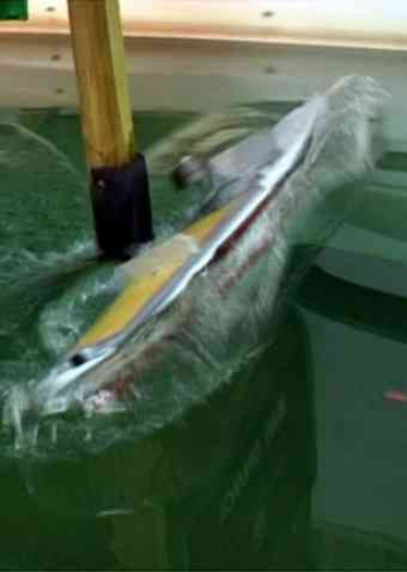
Figure 13. Narrow vessel, decked, 6 knots, 1.6 seconds after impact
